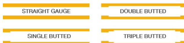
Figure 2 – Four different types of Frame Butting (2).
